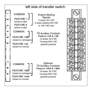
Figure 1-1. Connections to engine starting contact terminal block for 150 through 1200 amp. J & H–design transfer switches.
